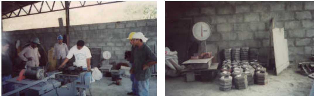
Picture 5.10: Block making machine and manufactured blocks
