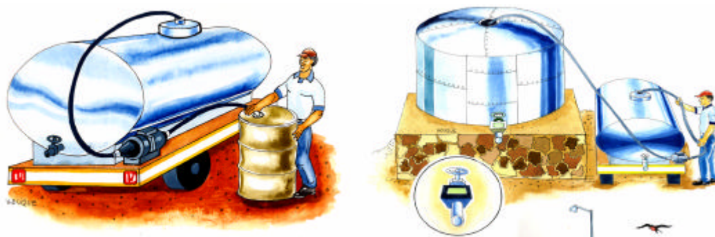
Picture 5.13: Special trailer for oil collection and temporary storage tanks
