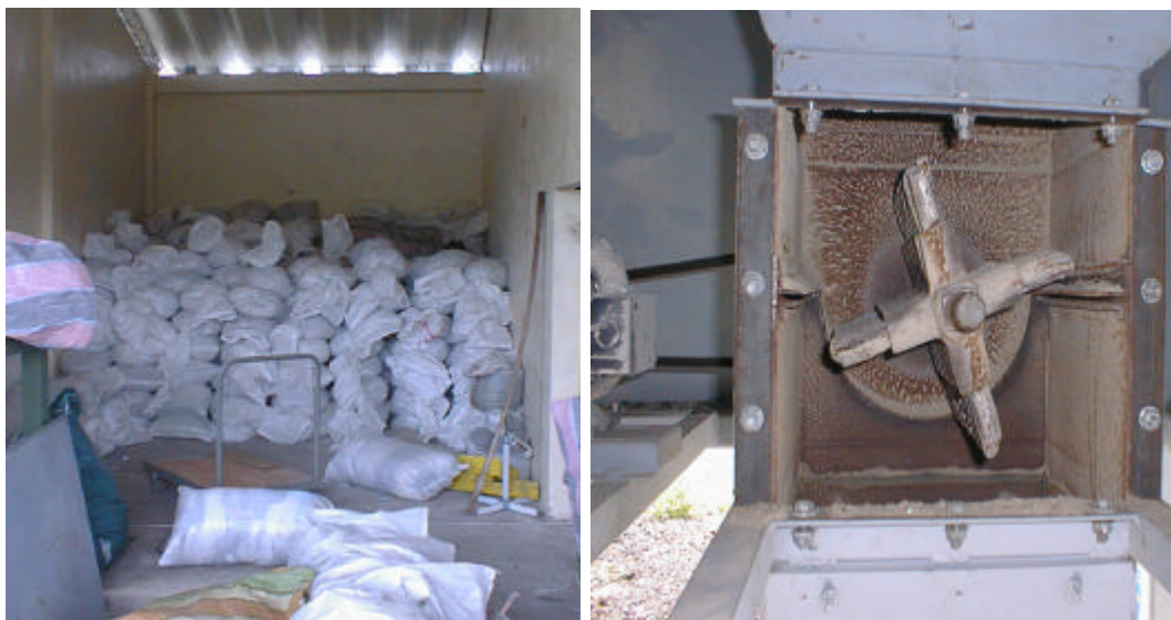
Picture 5.9: Storage of crushed glass and crushing mechanism
